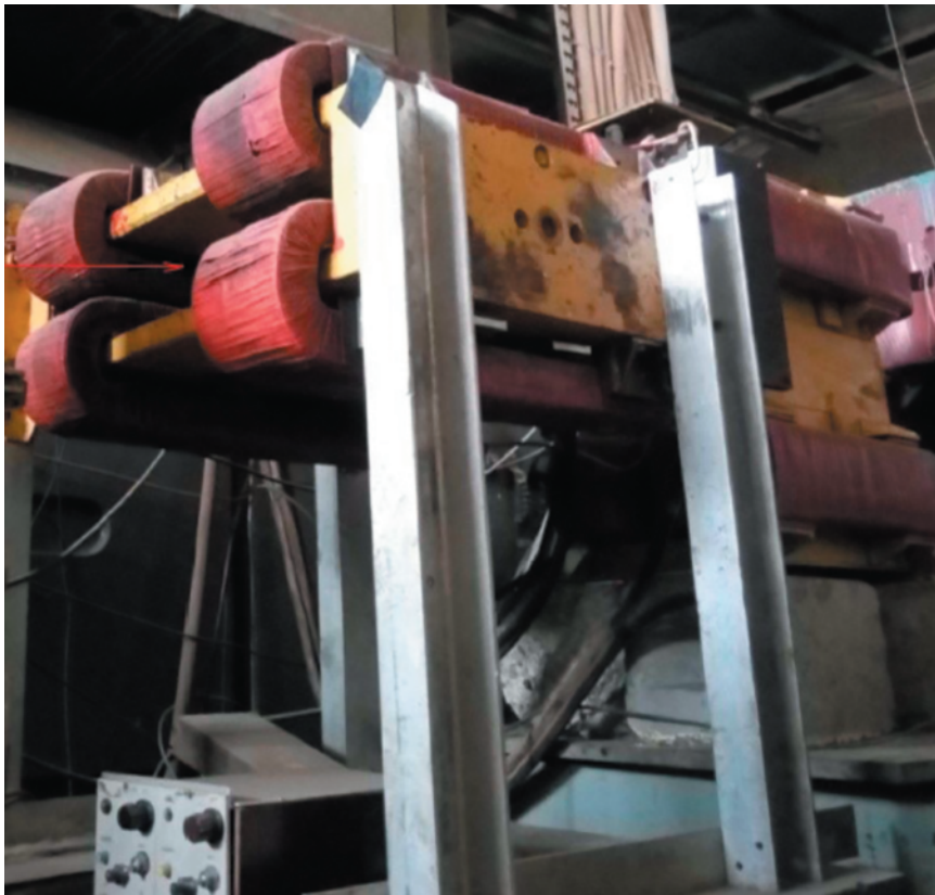
Fig. 9. The general form of the location of the KM1 and KM2 corrective magnets on channel no. 14 of U-70.
